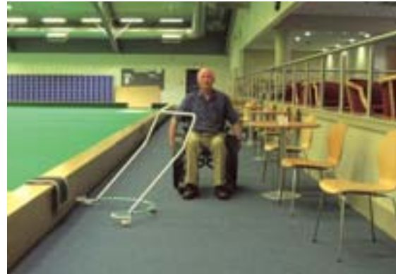
The green surrounds need to be wide enough for wheelchair access - see table on page 8
